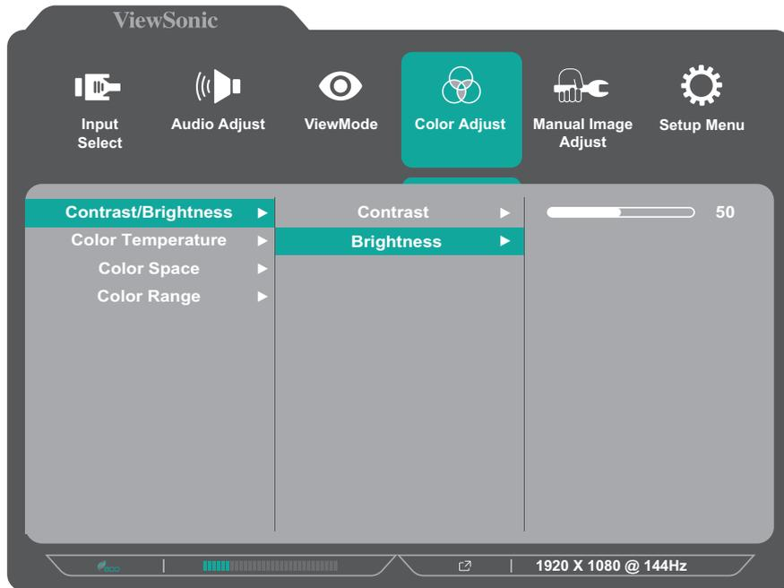
4. Press the **1(Shortcut)** or **2** key to adjust/select the setting. Then press the **3** key to confirm.
